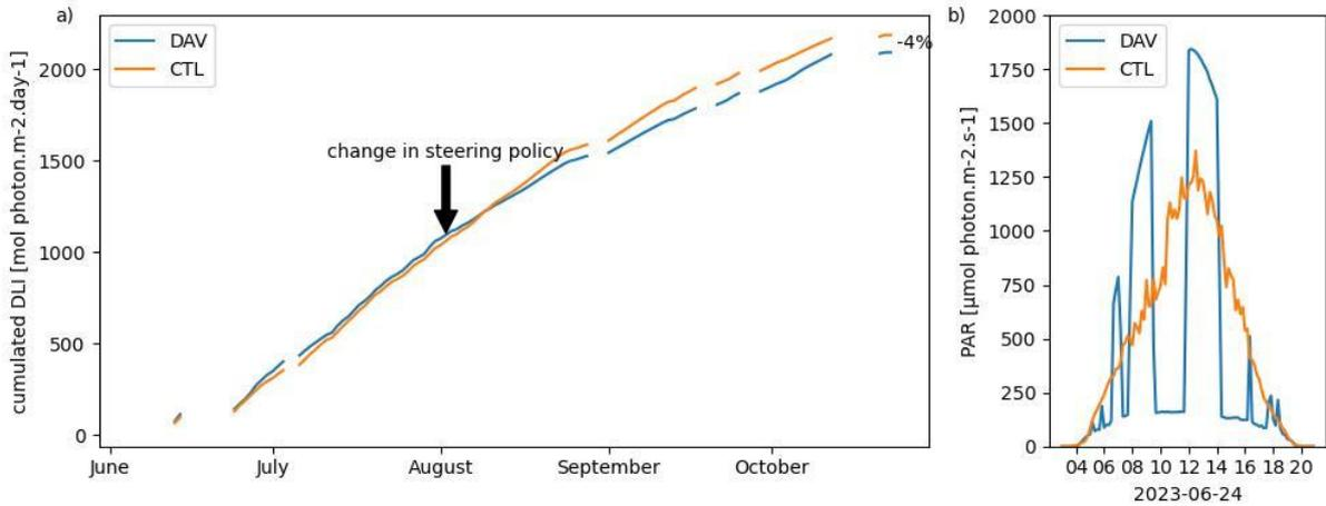
**Figure 2.** a) Cumulative daily light integral (DLI) for the 2023 growing season and b) Daily photosynthetically active radiation (PAR) for a typical clear summer day (2023-06-24) for dynamic agrivoltaic (DAV) and control (CTL). The arrow indicates a change in the steering policy.
