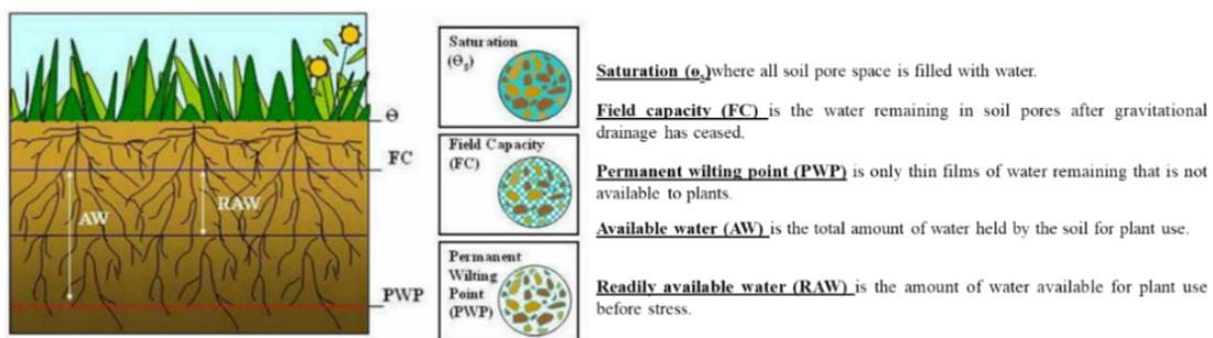
**Figure 1.** Diagram of water content in the root zone. Credits: D. Dukes et al., 2009 [5]
