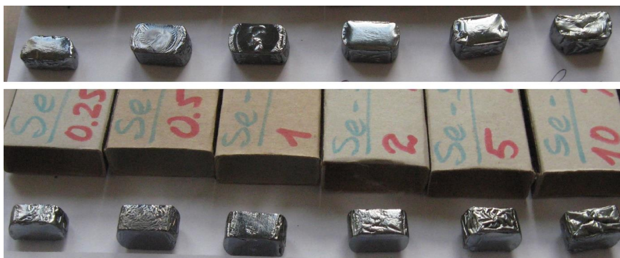
Figure 6. The samples of the Se-S series from the frontal (top) and lateral (bottom) view after the final cavitation treatment of 72°C.
