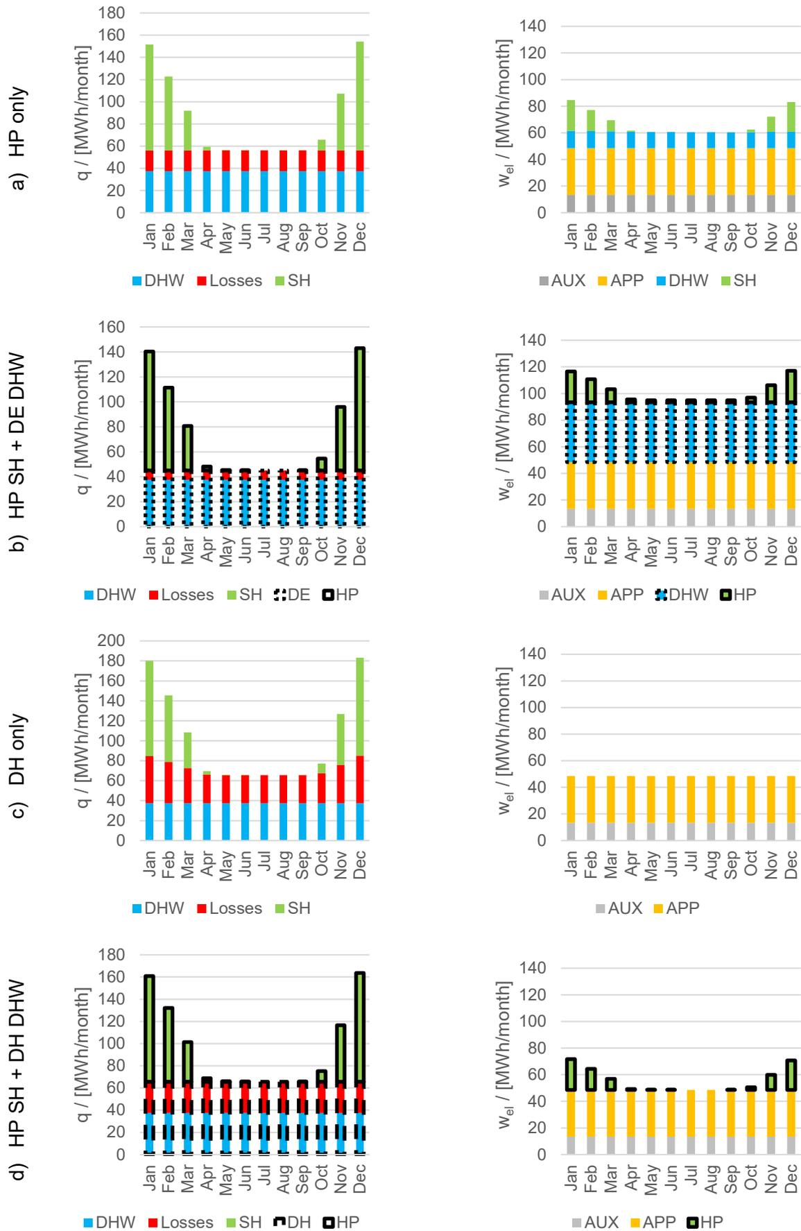
Figure 3: Monthly thermal (left) and electric (right) energy balance for the four investigated cases (a) – (d); APP = Appliances, AUX = Auxiliary
