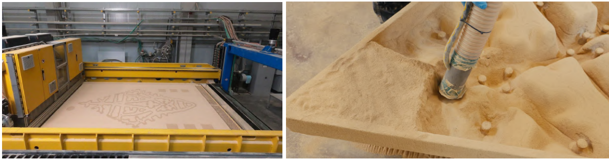
Figure 4. Left: Particle-bed printing of the full-scale (4 m) formwork, completed in 2 h 29 min. Right: Loose powder is vacuumed away and recycled, exposing the finished part.
