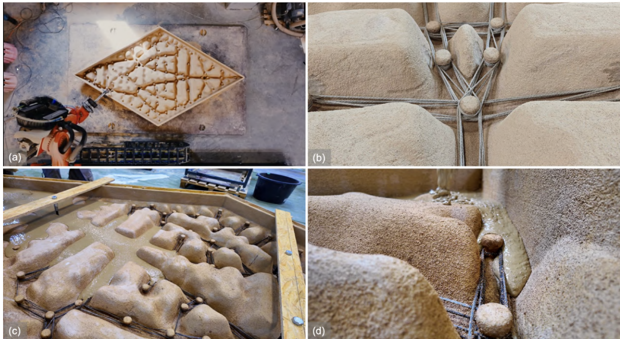
Figure 6. Fabrication sequence of the formwork: (a) after printing and loose powder is removed, a robot winds continuous flax fibres over the shell. The robot successfully negotiated congested node junctions without slippage or clearance issues (b); (c) once the fibres are epoxy-impregnated, a geopolymer is manually poured into the cavity; (d) the fluid mix flows readily through the formwork, leaving only negligible entrapped air.
