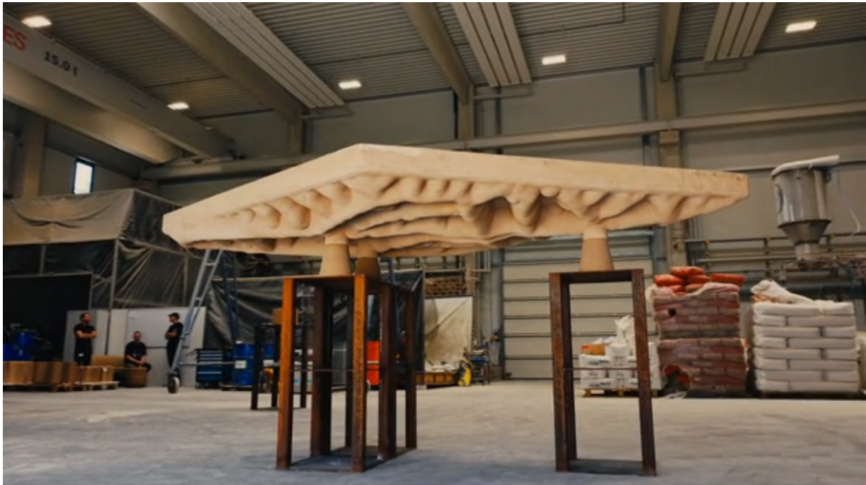
Figure 8. Completed 4 meter span prototype floor slab. The stay-in-place, 3D-printed formwork and the continuous flax-fibre winding now act as a single, integrated load-bearing system.
