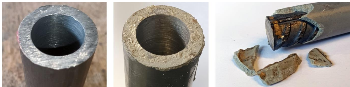
Figure 2. Reference socket before the pull-out test (left), after the pull-out test (middle), reinforcing bar bonded with UPAT UPM after the pull-out test from the reference socket (right)
