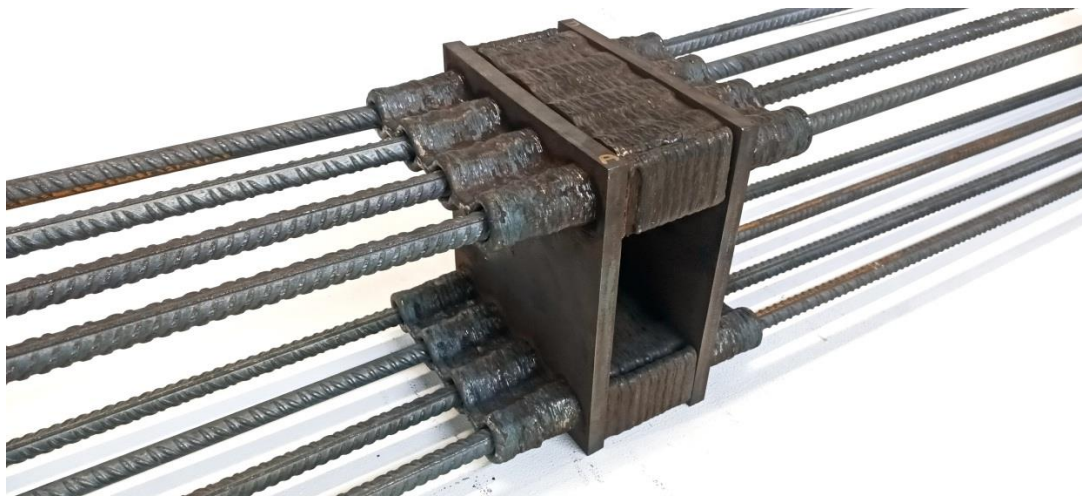
Figure 8. Real-scale test specimen for investigating the performance of WAAM-printed adhesive sockets for reinforcement connections
