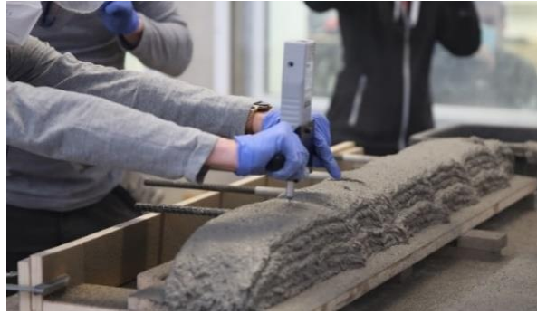
Figure 4. Testing of the printed specimen with a shotcrete penetrometer to obtain yield stress information.
