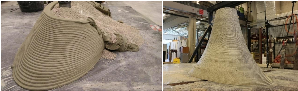
Figure 4. Failure during printing of the initial column design (left) and successful printing of the adjusted column design (right).
