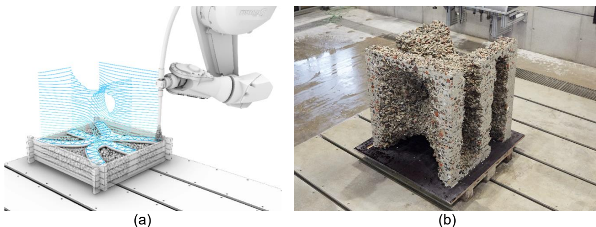
Figure 12: Large Particle 3D Concrete Printing LP3DCP: (a) Process schematic with indicated reinforcement inlay; (b) final demonstrator of one cubic meter of size. [29]
