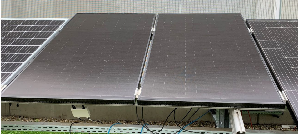
Figure 2. M1 and M2 (modules in the center) during Outdoor exposure with identically sized modules, mounted regularly on each other side
