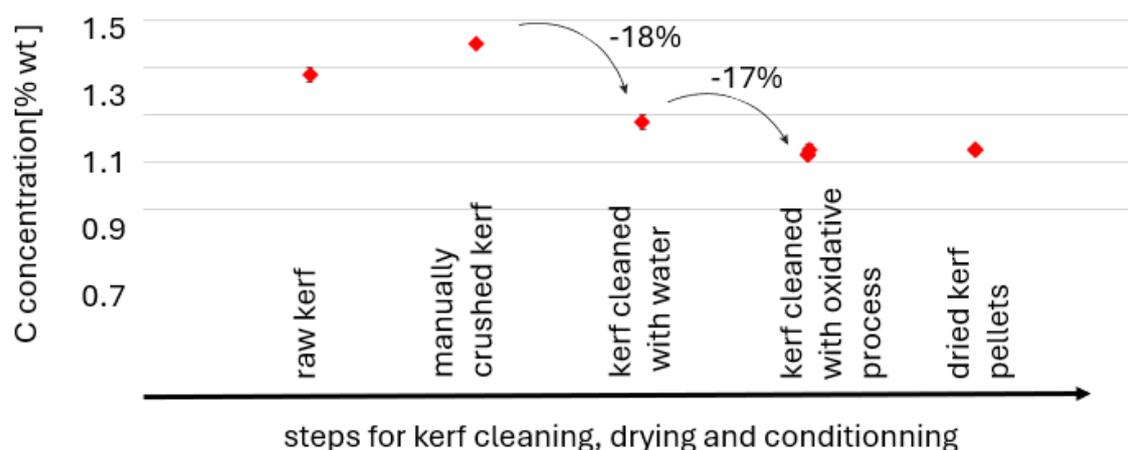
**Figure 2.** Carbon concentration in kerf sample after each process step
