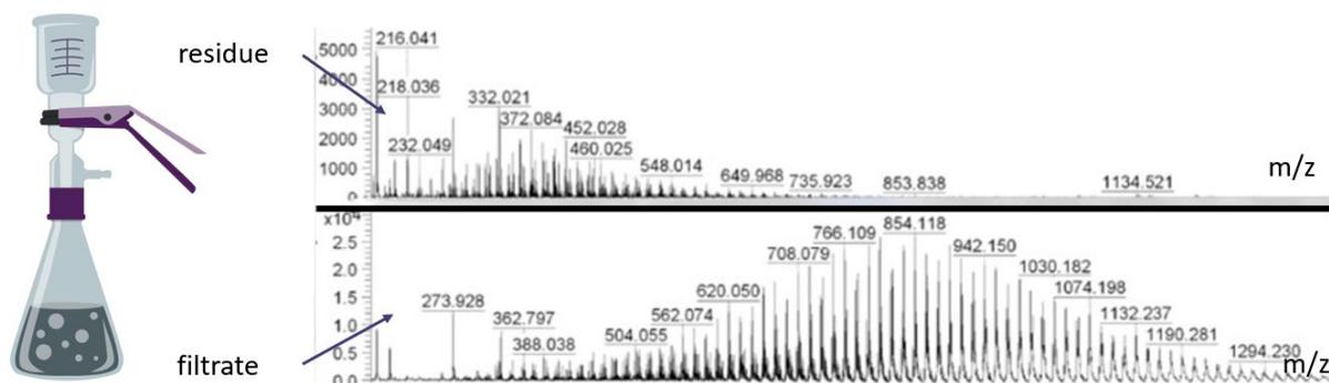
Figure 4. MALDI-TOF mass spectra of residue after filtration (top) and filtrate (bottom), respectively.
