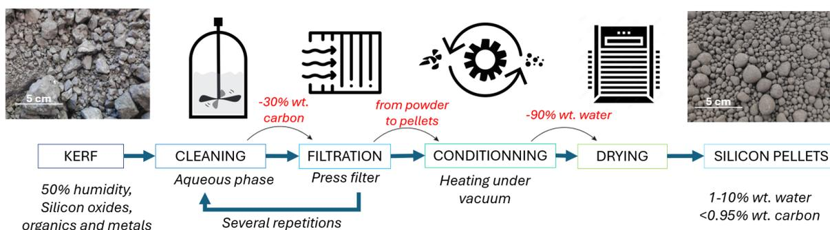
Figure 5. Global scheme of kerf cleaning, drying and conditioning processes
