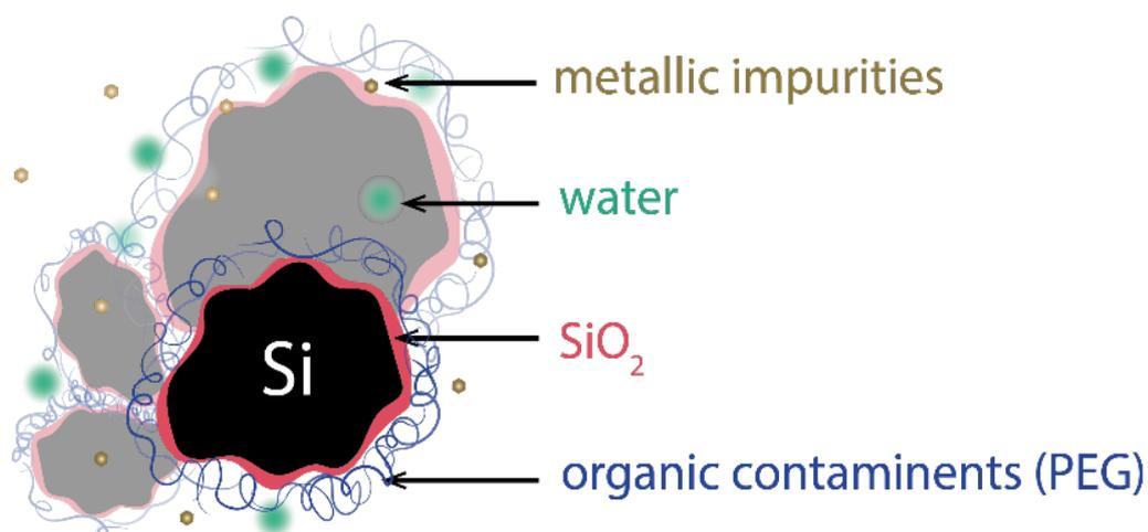
**Figure 1.** Schematic representation of kerf composition
