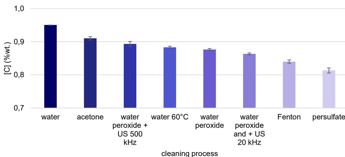
**Figure 3.** Carbon concentration in kerf samples after various oxidizing processes
