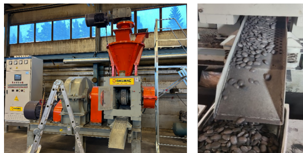
Figure 2. Briquetting process. DMSMAC briquetting machine and sample briquettes.
