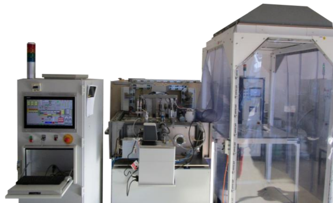
Figure 3. Photograph of the high-throughput PE-ALD prototype tool located at Plasma Electronic in Neuenburg am Rhein, Germany
