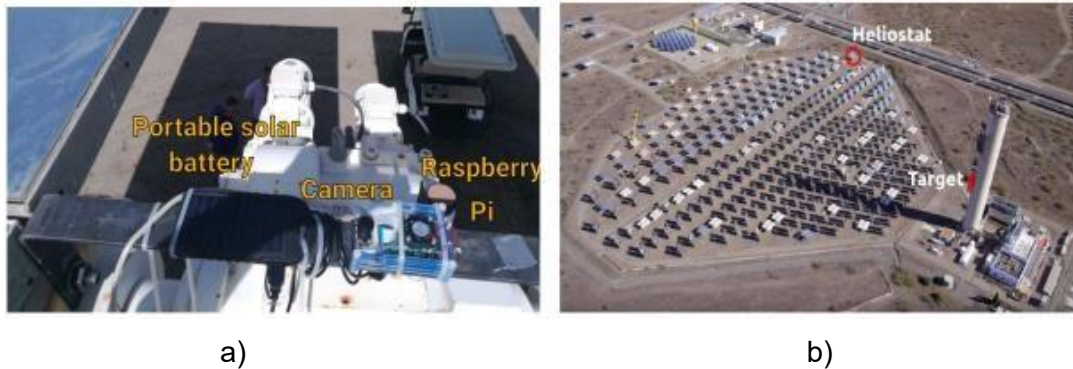
Figure 1. Smart solar tracker prototype (a) and selected installation in the CESA-I heliostat field at PSA (b).
