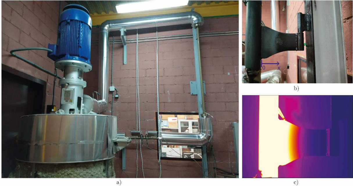
Figure 1. a) Photograph of the molten salt test loop. b) Detail of the clip. c) Thermal image of the clip
