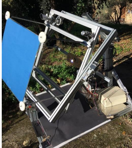
Figure 2. Photo of the test set up with the covered Fresnel lens mounted on the solar tracker
