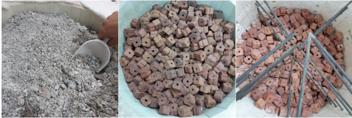
Figure 3. Left: material B after 1 charge-discharge cycle at set-point temperature 500°C and 4 cycles at 700 °C. Center and right: material A after several cycles at 700, 750, 800 and 850 °C. Picture on the center shows the upper of the storage tank and picture in the left.
