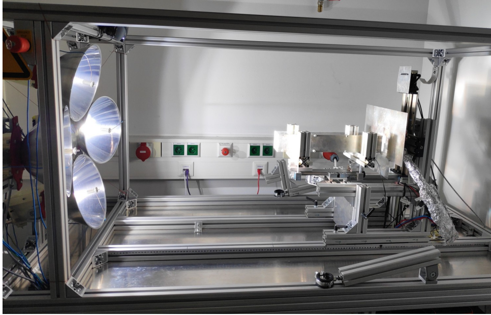
Figure 1. Photograph of the solar simulator during measurement. The four metal halide lamps and (elliptically shaped) reflector assembly (left) focus the light into the light guiding tunnel (LGT, centre right). On the opposite side of the tunnel (right) is a thermopile flux sensor mounted on an XY table, moving the sensor to measure the irradiance distribution.
