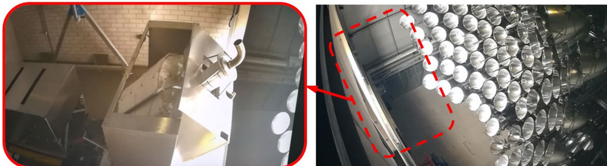
Figure 6. Odqa 100kW-scale solar thermal receiver tested in the tilted-axis configuration.
