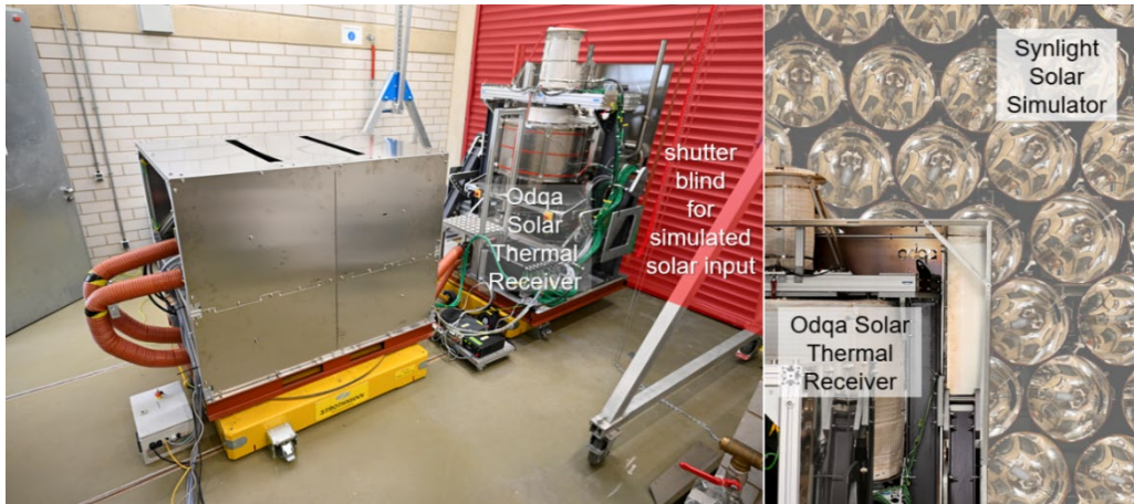
Figure 5. Odqa 100kW-scale solar thermal receiver mounted in front of the Synlight, DLR Jülich.
