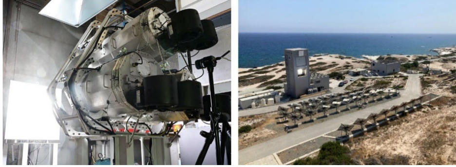
Figure 3. Left: Odqa 10kW-scale solar thermal receiver in-house solar simulator tests; right: heliostat field.
