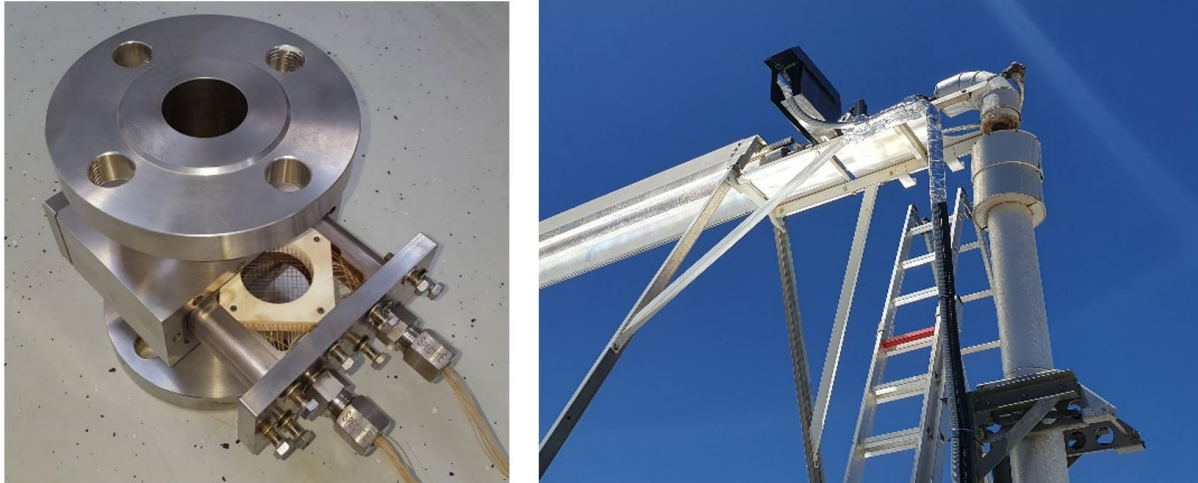
Figure 2. Photograph of WMS for JOSSI facility with ceramic inlay (left) and ready installed (right)
