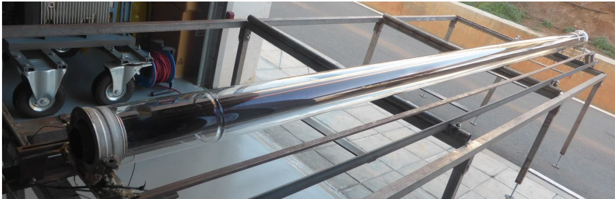
Figure 1. View of one of the PTR® 70 Gen 2 HCE tested.
