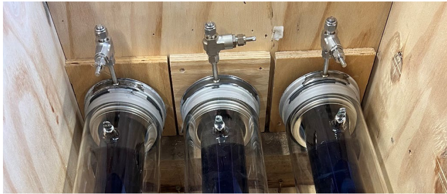
Figure 2. HCEs end sections after hydrogen doping at DLR. 8 mm pipes with valves and blind plugs mounted to the HCEs. (picture: DLR)
