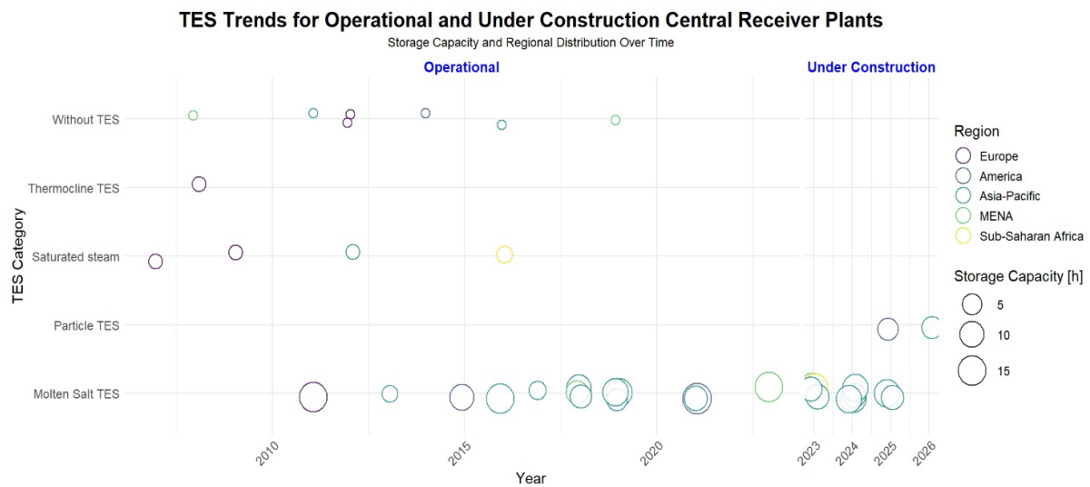
Figure 1. TES for operational and under-construction central receiver plants ordered chronologically by technology in color and capacity in point size (Data collected from NREL [6] and CSP.guru [20] databases).
