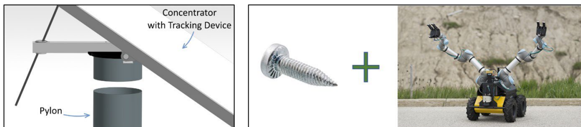
Figure 5. Components to be joined (left), vehicle with screwdriving robots (right)
