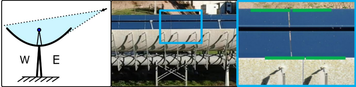
Figure 3. Module alignment measurement with edge detection. Images are taken by drone from positions that allow evaluation of alignment deviations along the collector row
