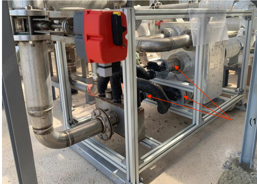
Figure 6. View of the equipment with the auxiliary heating systems assembled on it (1)
