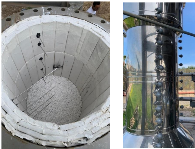
Figure 5. View of the inside of the tank (left) during assembly operations with the two rows of thermocouples visible and from the outside (right)
