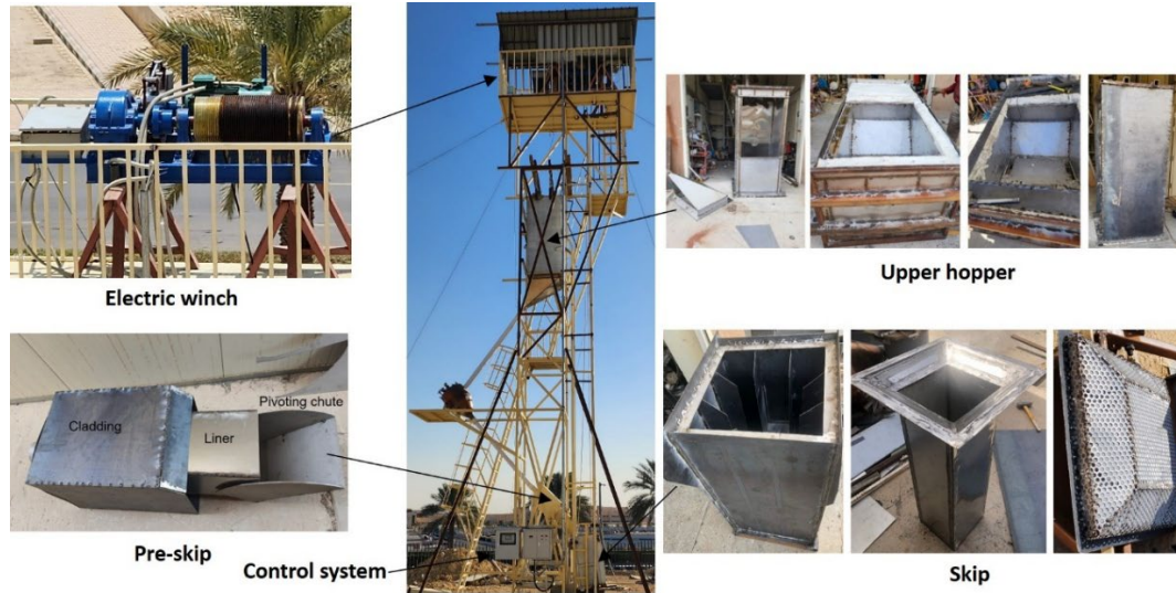
Figure 3. Skip-hoist PL during fabrication and after installation
