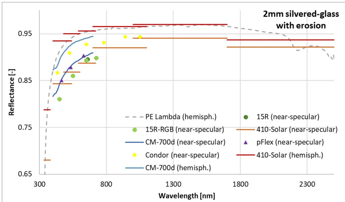
**Figure 4.** Reflectance spectra of 2 mm glass mirror after outdoor exposure, measured with all devices.
