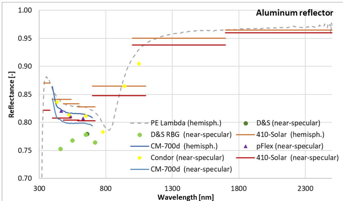
Figure 5. Reflectance spectra of aluminum mirror measured with all devices.
