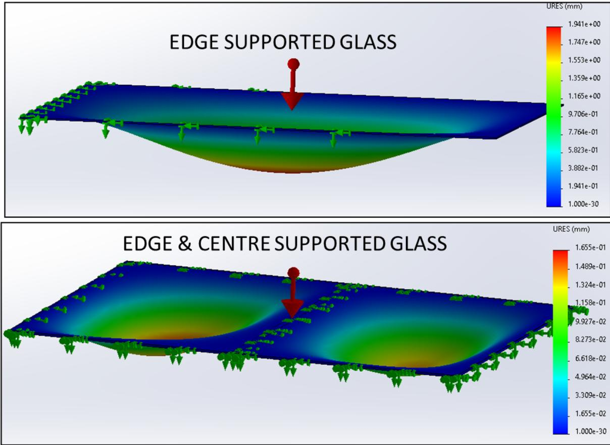
**Figure 6.** Deflection simulation results for 2850 X 2248 X 4mm glass mirror.
