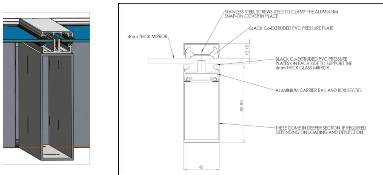
**Figure 5.** The glass heliostat mirror clamping system.
