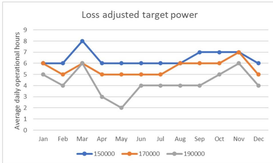
Figure 9. Expected Operating hours for the heliostat field (with a 2mm centre deflection).
