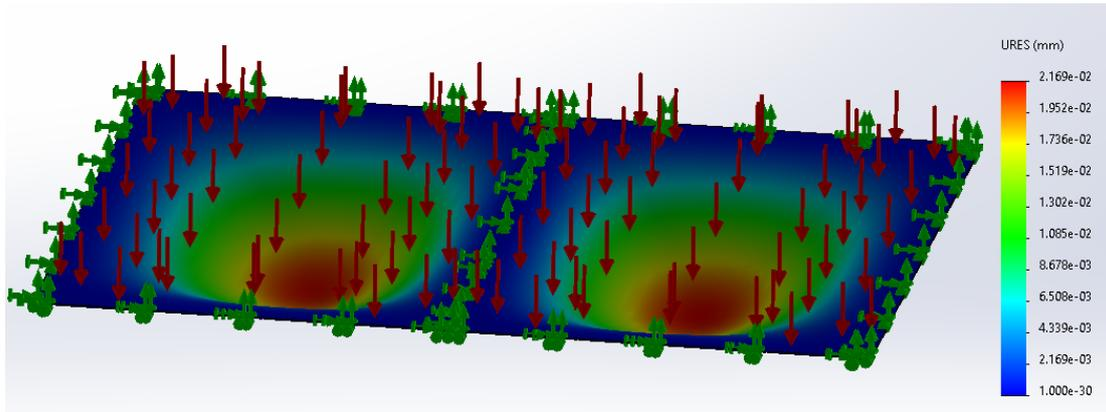
**Figure 8.** Wind load deflection simulation results for a dynamic wind pressure of  $15 \text{ N/m}^2$ .
