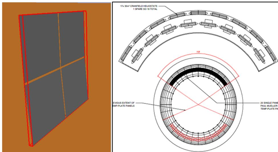
Figure 2. A single heliostat schematic (left) with an aerial view of the heliostat field (right).
