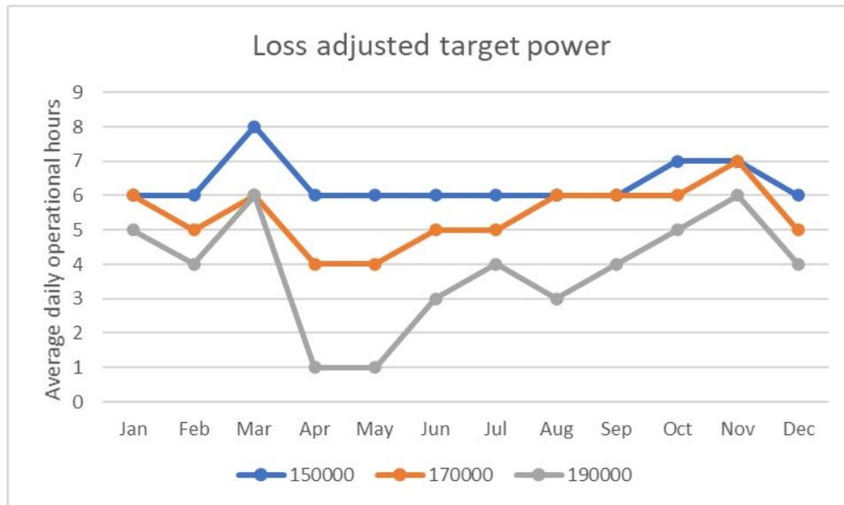
Figure 3. Expected Operating hours for the heliostat field.
