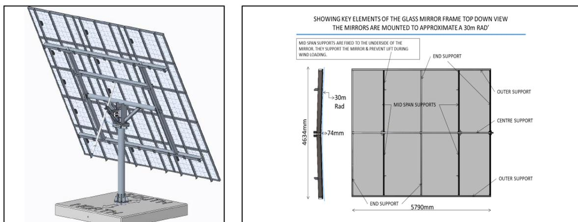
Figure 4. An overview of the structure of the novel heliostat and its constituent parts.
