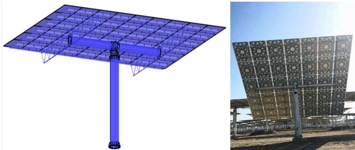
**Figure 2.** A 3D model (left) and an actual picture (right) of the heliostat
