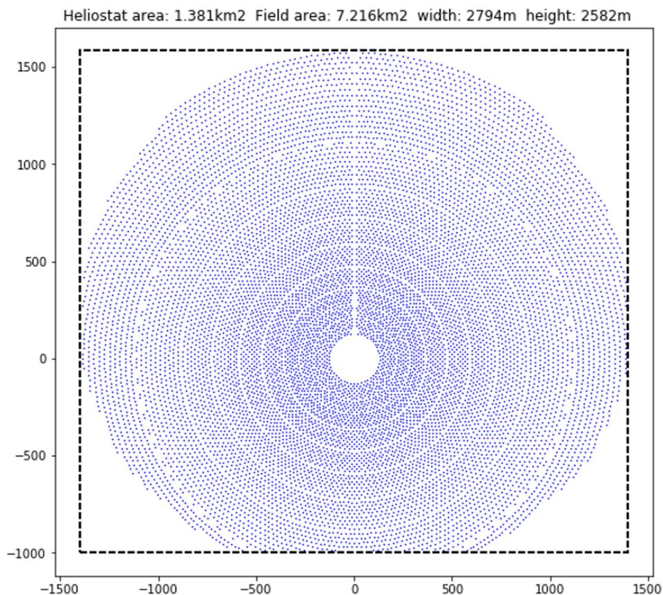
**Figure 3.** The layout of the solar field
