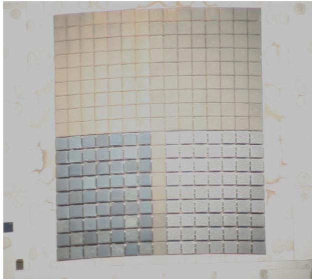
**Figure 2.** Final testing configuration of SolAir 3000 receiver including state-of-the-art absorber modules (upper half) and new developed absorbers (bottom half)
