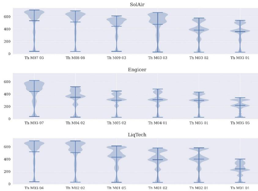
**Figure 4.** Probability density graphs of the test temperatures (in °C) for the three different absorber designs tested (July, 26th).
