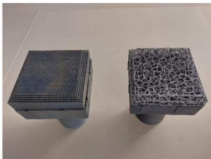
**Figure 1.** Samples of the new generation of volumetric absorbers developed into the NEX-TOWER project
