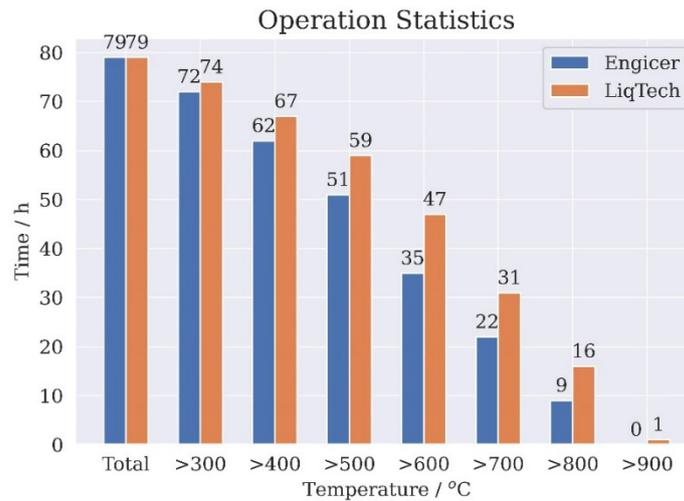
**Figure 3.** Operation statistics of new absorber cups installed on the Solair3000 receiver.
