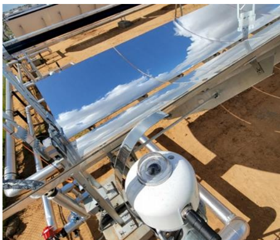
Figure 7. Tracking pyranometers. The shadow band is seen in the foreground.
