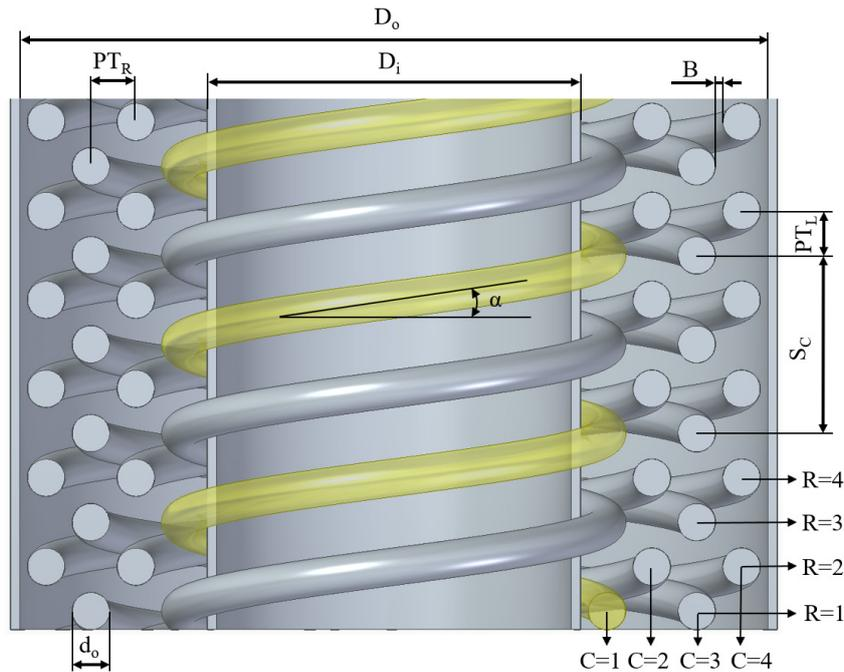
**Figure 3.** Coil-Wound Heat Exchanger geometrical parameters
