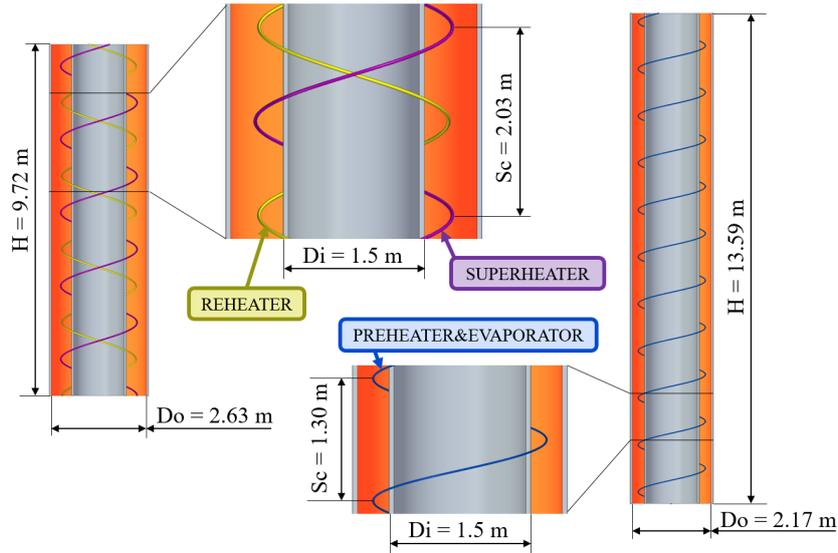
Figure 4. Geometrical results of the steam generator system.
