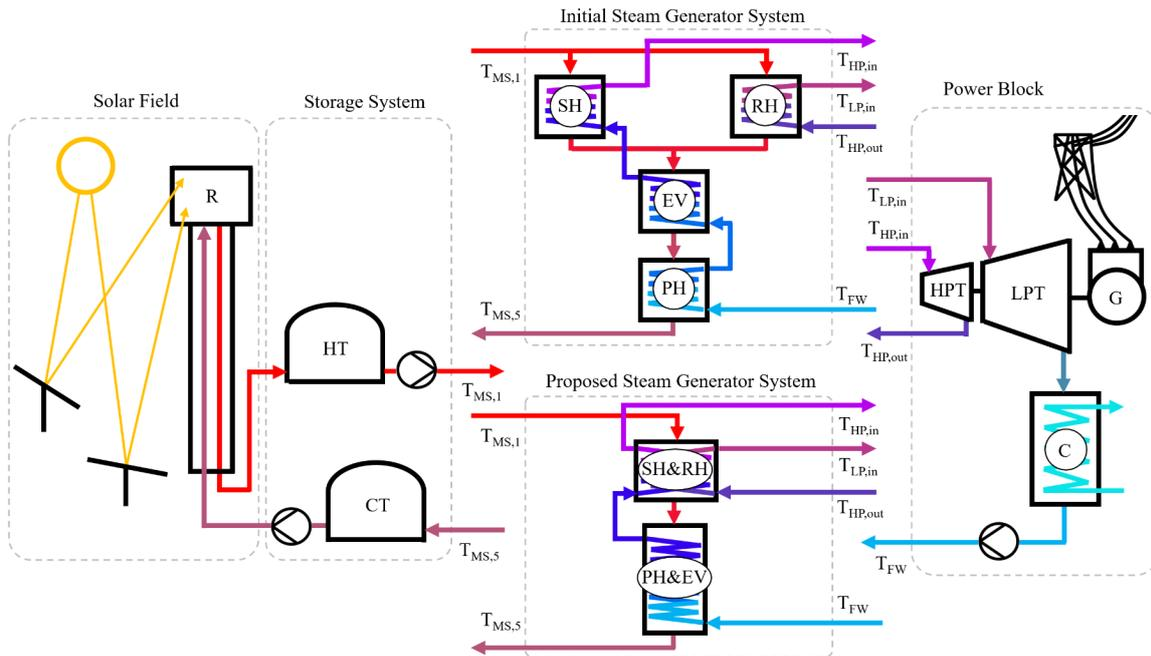
**Figure 1.** Initial and proposed steam generator system comparison in a solar tower plant
