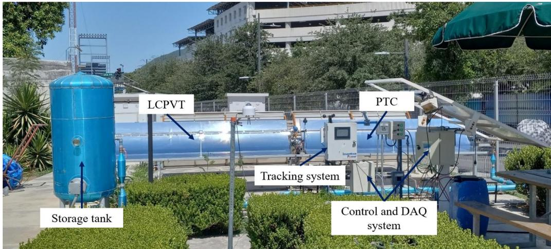
**Figure 2.** LCPV-T performance testing.
