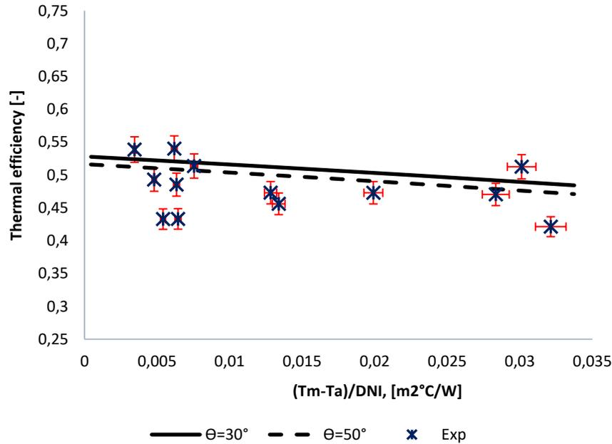
Figure 4. LCPVT instantaneous thermal efficiency (theoretical vs. experimental).
