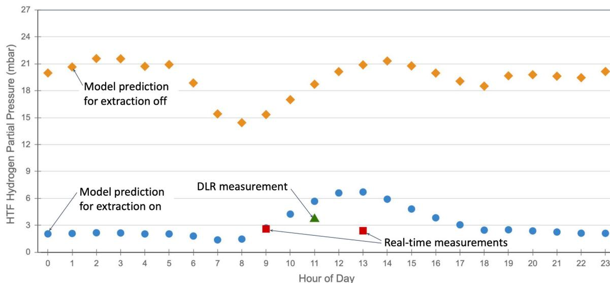
**Figure 6.** Expansion vessel headspace gas hydrogen measurements and modeled data
