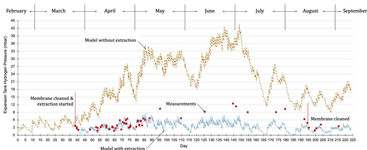
Figure 7. Headspace gas hydrogen measurements and modeled data for 2023
