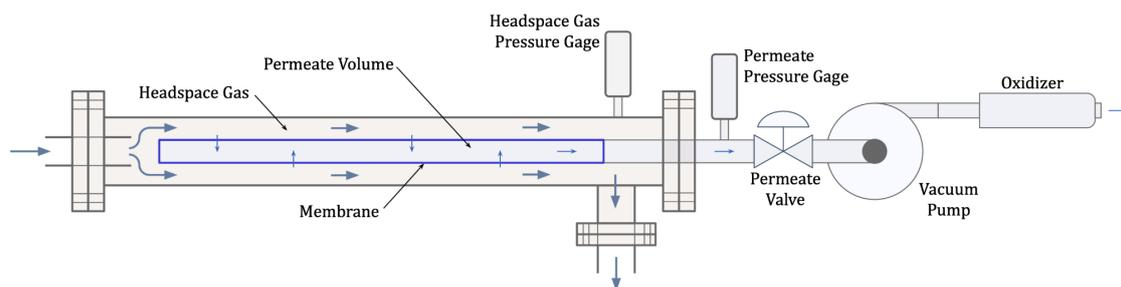
Figure 2. Integrated sensor/separator design that was installed at the NSO power plant
