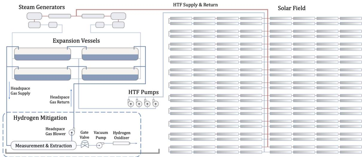
**Figure 1.** Hydrogen mitigation process interface with the power plant expansion tanks
