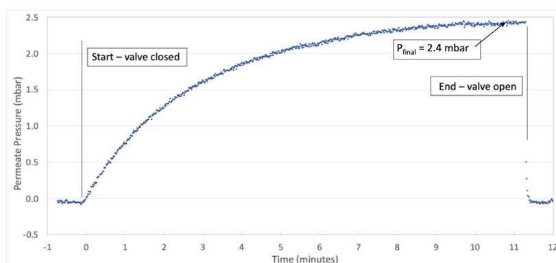
**Figure 4.** Permeate pressure versus time for measuring hydrogen in headspace gas
