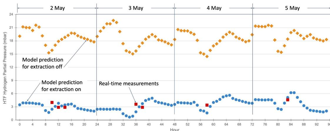
**Figure 5.** Expansion vessel headspace gas hydrogen measurements and modeled data
