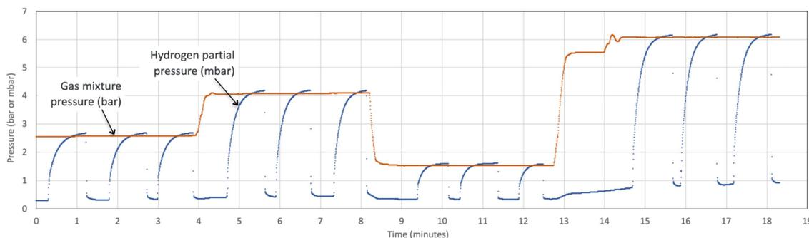
Figure 3. Permeate-volume pressure response in separation and sensing modes
